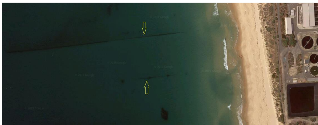
Figure 3. An example of a coastal outfall for Christies Beach WWTP, South Australia.
